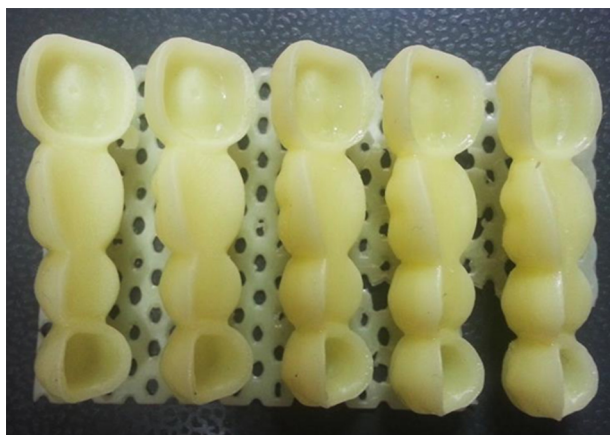
Fig. 4. Polymer temporary bridges, produced by stereolithography.
